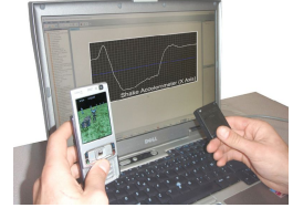
Fig. 3. OIDE Debugging and Logging tools. In the example, the Shake accelerometer events are logged in order to tune the interaction with the mobile game.
